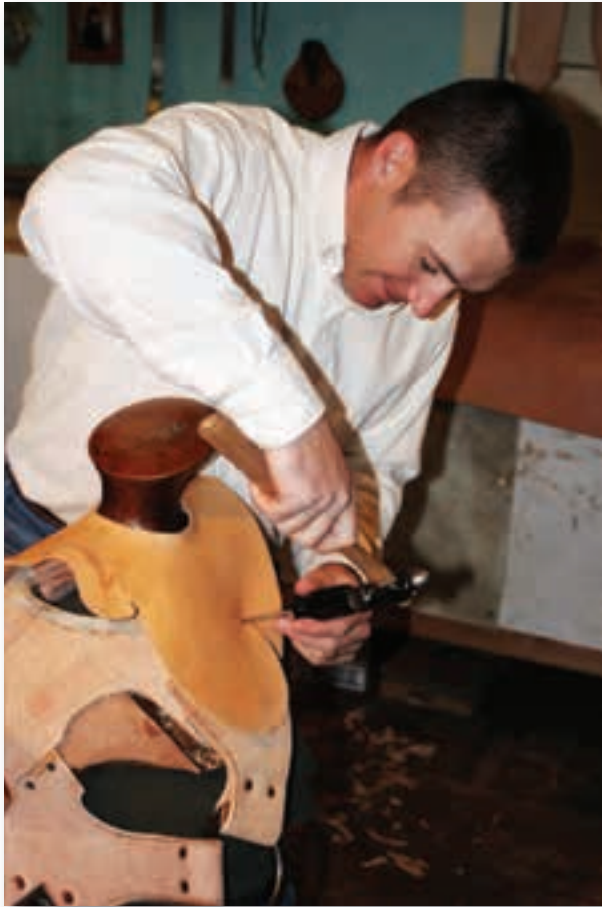
While installing a fork cover on a Wade saddle, Matt works on taking the stretch out of the leather for a tight fit.
