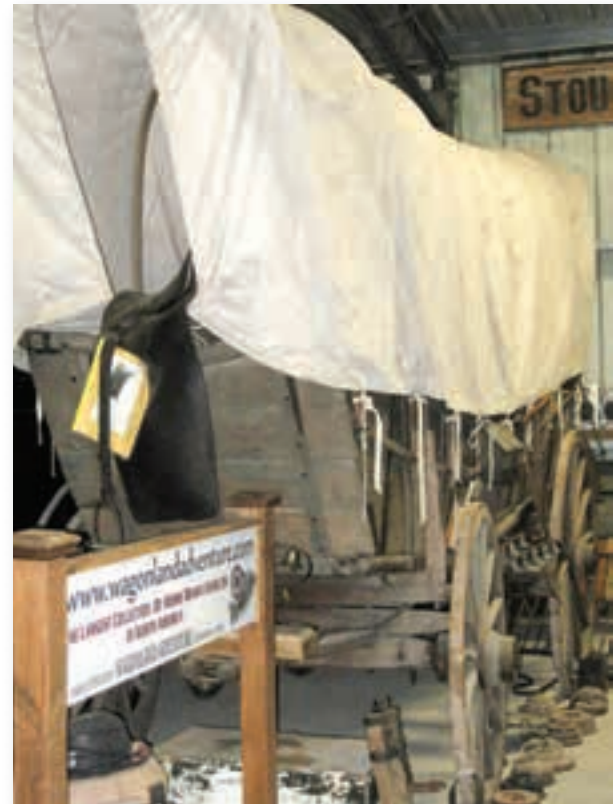
The legendary Conestoga wagon with its curved floor and flared ends could haul up to six tons of freight.
